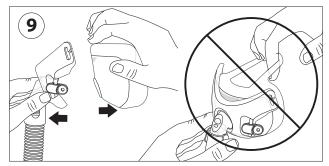
4. Quick Release Tube - Squeeze the quick release tabs. Pull the tube away from the mask frame 10.
